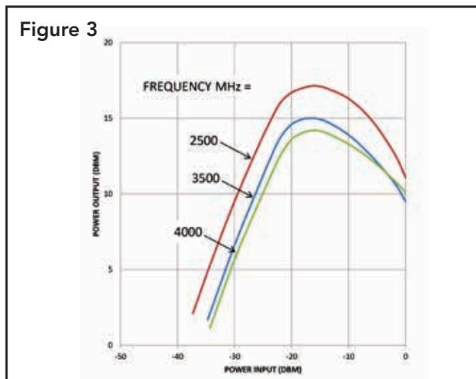
The gain is essentially constant at a given frequency for low RF drive levels, but decreases at higher levels. When the RF electric field becomes too strong, as a result of either amplification or input signal, the amount of energy which the beam can deliver to the wave reaches a maximum limit. This condition, known as the saturation point of the TWT, represents the maximum power which can be delivered for a given condition of beam current. If the input power is increased beyond the value which
